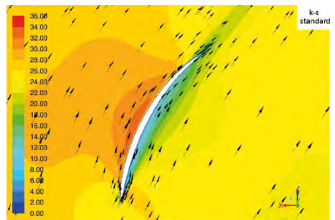
Contours and velocity vectors around the blade for the turbulence model
